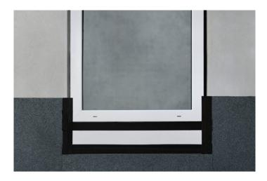
In the event of installation with the blaugelb Trio**therm**\* Pre-Wall Installation System, the blaugelb Foil Outside **SL**<sup>1050</sup> Power One 75 mm also has to be installed in the inner corners at the side and bottom connection of the blaugelb Trio**therm**\* Profiles to the wall components.
