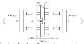
Our blaugelb Anti-Panic Square Pins generally contain two dimensions in the name. The first of these is the interior dimension (SI) and the second is the exterior dimension (SA).
